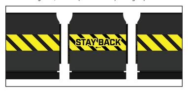
Insert Vertical bars (long bar) in both, right and left, pockets of the Center panel
